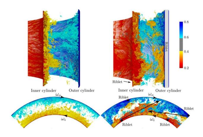
Turbulent Taylor-Couette flow, without surface roughness (images on the left, side and top view), and with roughness/riblets. Credit: University of Twente
