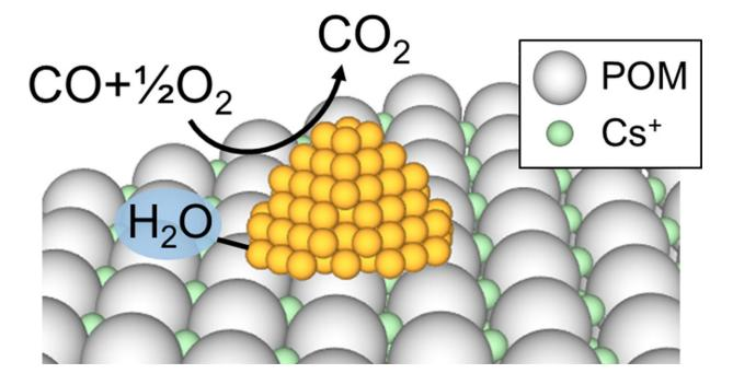
New catalyst consisting of gold nanoparticles supported on a Keggin-type polyoxometalate (POM) with a cesium salt. The structure showed high activity and stability for CO oxidation; trace amounts of water were found to be essential to the function of the material. Catalytic activity showed a unique, U-shaped dependence on temperature. Credit: Toru Murayama
