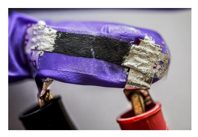
University of Washington graduate student, Jinyuan Zhang, demonstrates how a wearable sensor can measure finger pressure. Credit: Dennis R. Wise/University of Washington
