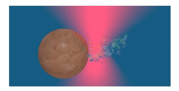
Going in circles. A micrometer-sized silica sphere with irregular iron oxide inclusions is trapped by optical tweezers (red area indicates focused laser light). Heating of the sphere by the light causes a near-critical liquid mixture to develop local concentration variations (trailing bubbles) that push the sphere to revolve around the beam. Credit: F. Schmidt/Univ. of Gothenburg
