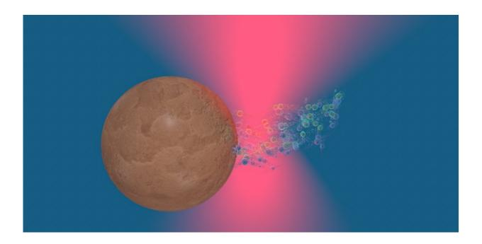
Going in circles. A micrometer-sized silica sphere with irregular iron oxide inclusions is trapped by optical tweezers (red area indicates focused laser light). Heating of the sphere by the light causes a near-critical liquid mixture to develop local concentration variations (trailing bubbles) that push the sphere to revolve around the beam. Credit: F. Schmidt/Univ. of Gothenburg
