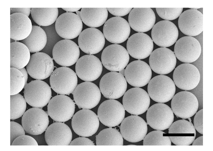
The method that the Illinois engineers developed allows them to make tiny, uniform capsules and control the size, allowing for a capsule-within-a-capsule technique. Credit: Kevin Kim
