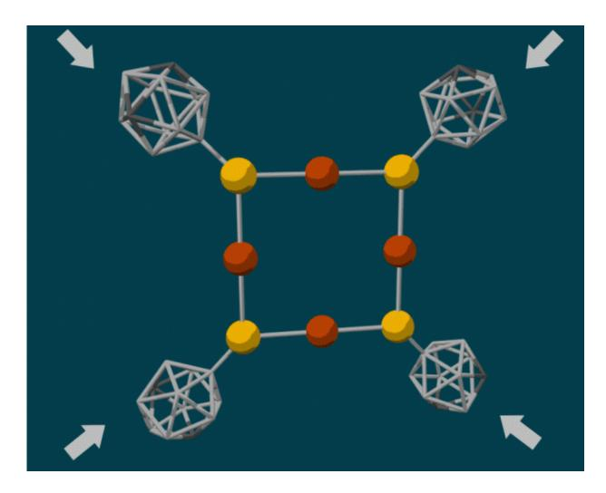
An animation shows how attaching molecular anvils (gray cages) to softer molecules (red and yellow balls) distributes the pressure from a bigger diamond anvil unevenly, so chemical bonds bend and eventually break around the atom that bears the largest deformation (circled red ball). Credit: Greg Stewart/SLAC National Accelerator Laboratory
