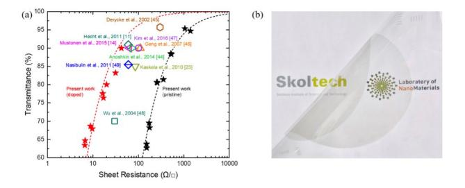
(a) Comparison of the performance of films based on single-walled carbon nanotubes after p-type doping: sheet resistance vs. optical transparency in the visible range. Dashed lines indicate theoretical relationship between transmittance and sheet resistance of pristine (black) and doped SWCNT films (red) obtained in this work. (b) A photograph of a doped single-walled carbon nanotubes film on a flexible PET substrate. Credit: Skolkovo Institute of Science and Technology
