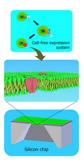
Cell-free ion channels embedded in bilayer lipid membranes formed in silicon chips. Credit: Ayumi Hirano-Iwata
