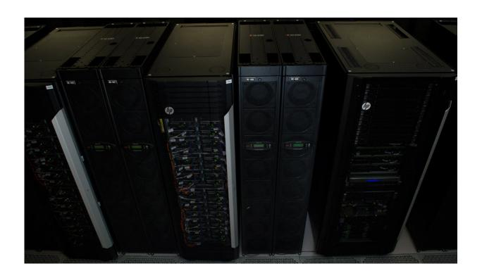
The Maverick supercomputing system at the Texas Advanced Computing Center. Maverick is an XSEDE-allocated dedicated visualization and data analysis resource architected with 132 NVIDIA Tesla K40 "Atlas" GPU for remote visualization and GPU computing to the national community. Credit: TACC
