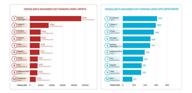
TOP500 LINPACK and HPCG charts of the fastest supercomputers of 2017. The rearranged order and drastic reduction in estimated speed for the HPCG benchmarks are the result of a different method of testing modern supercomputer programs. Credit: Sandia National Laboratories
