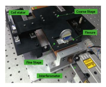
An integrated nanopositioning device can achieve high precision with a simpler and less expensive design than typically used. Credit: IEEE. Reprinted, with permission, from Ref 1.
