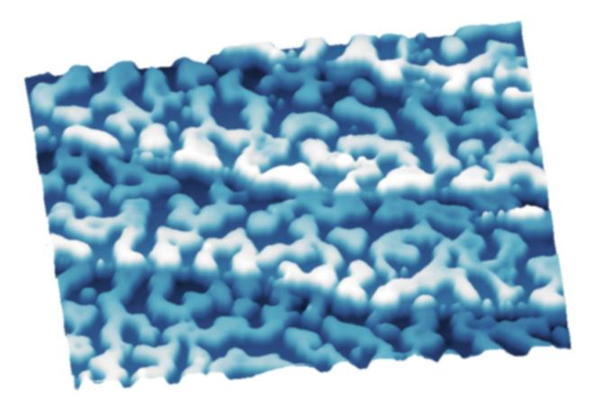
Island structures, visible after breaking the crystal. Credit: TU Wien
