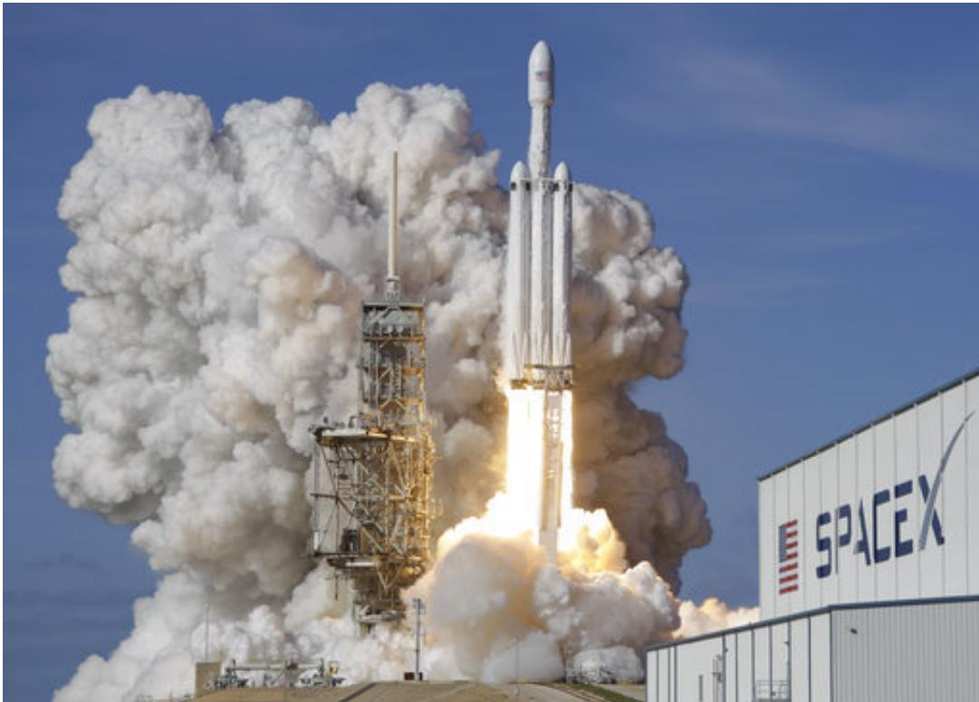
A Falcon 9 SpaceX heavy rocket lifts off from pad 39A at the Kennedy Space Center in Cape Canaveral, Fla., Tuesday, Feb. 6, 2018. The Falcon Heavy, has three first-stage boosters, strapped together with 27 engines in all. (AP Photo/John Raoux)
