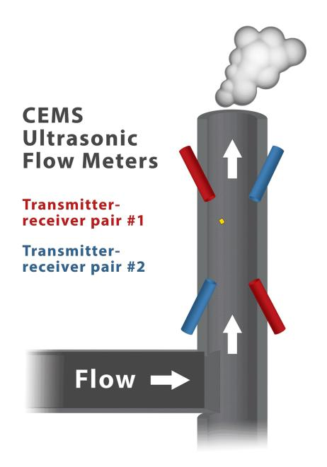
Two pairs of CEMS ultrasonic flow meters arranged in an x-pattern installation. Credit: National Institute of Standards and Technology
