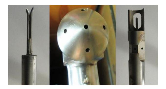
Three types of pitot probes. From left to right: s-probe, spherical probe, prism probe. Credit: National Institute of Standards and Technology
