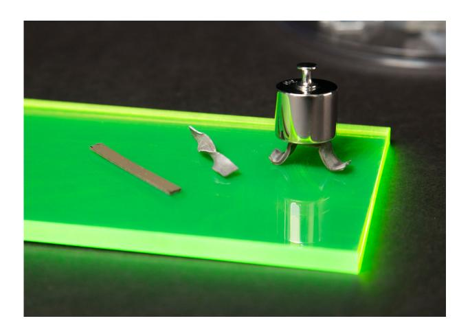
Examples of the new smart material, left to right: A flexible strip; a flexible strip that stiffened when twisted; a flexible strip transformed into a hard composite that can hold up a weight. Credit: Christopher Gannon/Iowa State University
