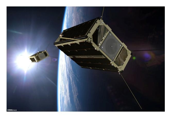
ESA's biggest small satellite yet: the GomX-4B six-unit CubeSat will demonstrate miniaturised technologies, preparing the way for future operational nanosatellite constellations. Credit: GomSpace
