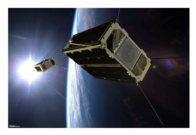
ESA's biggest small satellite yet: the GomX-4B six-unit CubeSat will demonstrate miniaturised technologies, preparing the way for future operational nanosatellite constellations. Credit: GomSpace
