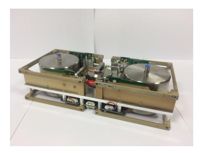
GomX-4B's cold-gas thruster system takes up two half-CubeSat units at one side of the nanosatellite, with two spherical titanium tanks filled with liquid butane. It has four 1 mN thrusters, typically to be fired in pairs while keeping one set in reserve. Credit: Nanospace
