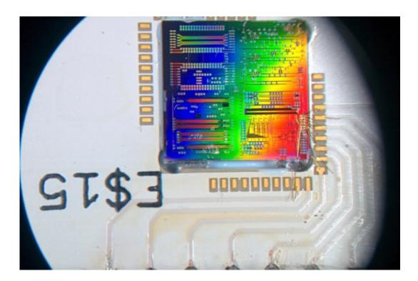
Microscope image of a silicon chip that contains tens of quantum optics experiments. The newly developed detector is tiny: it occupies less than 1 mm2 on the chip shown, in the bottom right. Credit: University of Bristol
