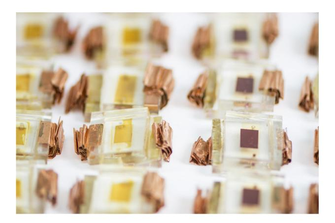
In studies on the ageing of perovskite solar cells and the dye cells in the picture, a sufficiently large number of samples is one of the prerequisites for quality. Credit: Valeria Azovskaya, Materials Platform, Aalto University
