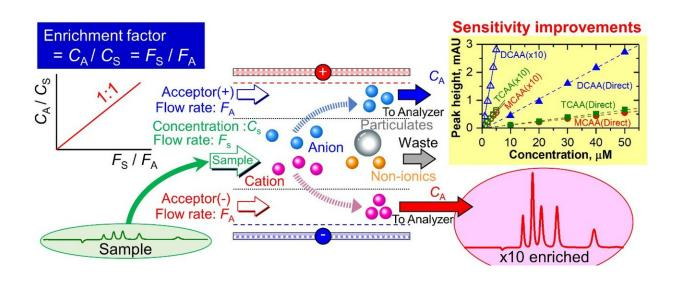
To increase the detection sensitivity of ionic solutes in a water sample, it is enriched via electrodialytic ion transfer before it passes to the analyzer. [Reprinted from Talanta, 180, Shin-Ichi Ohira, Takayuki Yamasaki, Takumi Koda, Yuko Kodama, and Kei Toda, Electrodialytic in-Line Preconcentration for Ionic Solute Analysis, 176-181, (April 2018) with permission from Elsevier. doi: 10.1016/j.talanta.2017.12.054] Credit: Dr. Shin-Ichi Ohira
