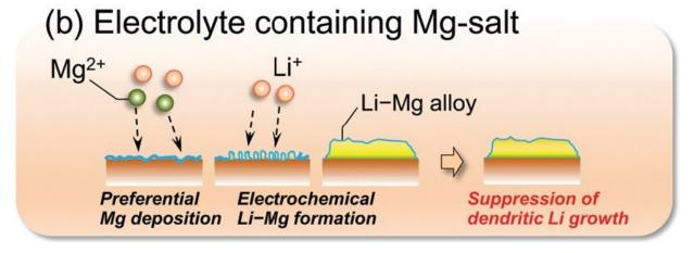
Schematic illustration of the proposed suppressing effect of Li dendritic growth by addition of Mg-salt. Credit: Royal Society of Chemistry
