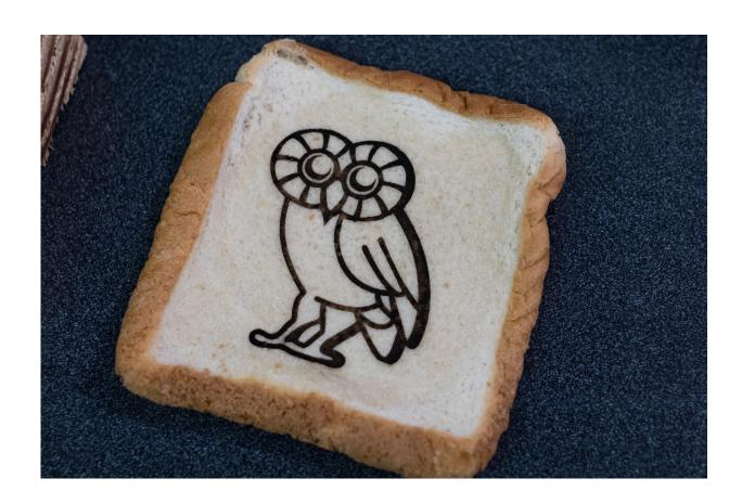
Laser-induced graphene is a highly conductive addition to a piece of bread. A Rice University lab is using an industrial laser to write graphene patterns on everyday objects, including food, cloth, cardboard and wood. Credit: Jeff Fitlow/Rice University
