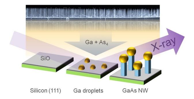
Schematic of the experiment: Fueled by a stream of gallium atoms and arsenic molecules, nanowires grow beneath gallium droplets on a silicon wafer. The growth process can be monitored live with X-rays. The fully grown nanowires were then investigated with an electron microscope (background image). Credit: KIT, Philipp Schroth
