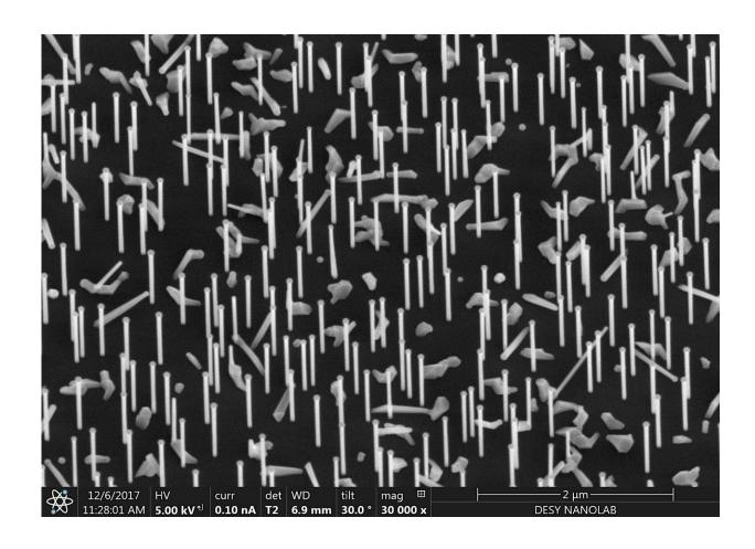
Nano forest: 'Aerial' view of the tiny wires growing on a silicon wafer, captured with a scanning electron microscope at the DESY NanoLab. Credit: DESY, Satishkumar Kulkarni/Thomas Keller
