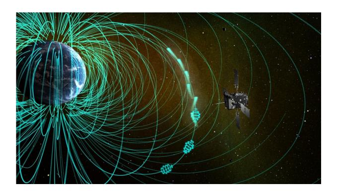
The ERG spacecraft observed chorus waves and scattered electrons in the magnetosphere, the origin of pulsation auroras. The scattered electrons precipitated into the atmosphere resulting in auroral illumination. Intermittent occurrence of chorus waves and associated electron scattering lead to auroral pulsation. Credit: 2018 ERG science team.
