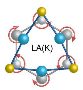
This diagram maps out atomic motion in separate phonon modes. At left ("LO" represents a longitudinal optical mode), selenium atoms exhibit a clockwise rotation while tungsten atoms stand still. At right ("LA" represents a longitudinal acoustic mode), tungsten atoms exhibit a clockwise rotation while selenium atoms rotate in a counterclockwise direction. Credit: Hanyu Zhu, et al
