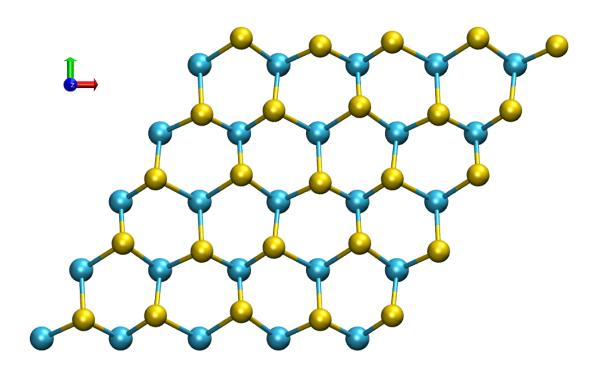
The atomic motion in a 2-D material, tungsten disulfide, is shown in this animation. In this phonon mode (known as longitudinal optical mode or LO), the selenium atoms (yellow) rotate clockwise while the tungsten atoms (blue) are still. Credit: Hanyu Zhu, et al
