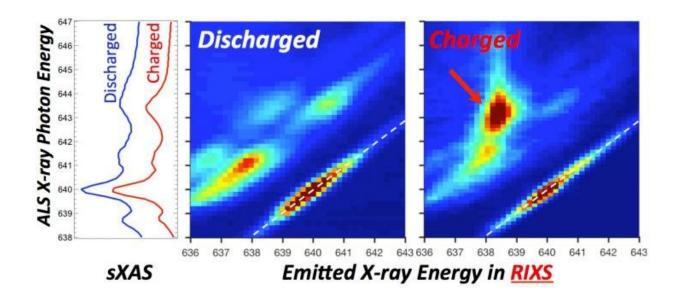
In the middle and right images, produced using an X-ray technique at Berkeley Lab, there is a clear contrast in an exploration of the manganese chemistry in a battery electrode material. Another technique, known as sXAS (graph at left) does not reveal the same level of contrast. Credit: Berkeley Lab
