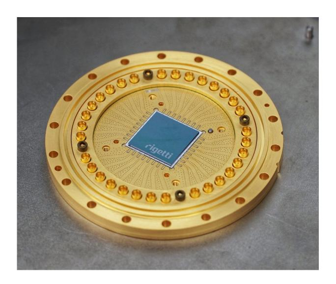
Rigetti's 19Q superconducting quantum processor. Credit: Rigetti Computing
