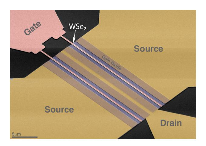
False-colored scanning electron microscope (SEM) image of a radio-frequency field-effect transistor (RF-FET) composed of a 2-3 layer-thick epitaxially-grown tungsten diselenide (WSe2) active channel. Credit: Brian Bersch/Penn State
