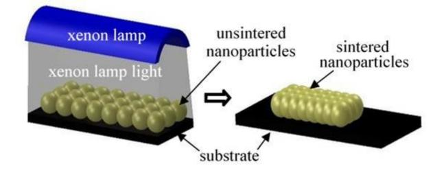
Fusing, or sintering, nanoparticles by exposing them to pulses of intense light from a xenon lamp. Credit: Rajiv Malhotra/Rutgers University-New Brunswick
