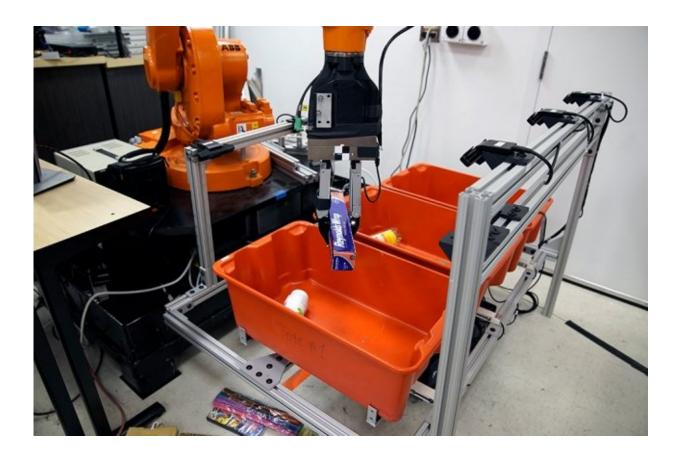
The "pick-and-place" system consists of a standard industrial robotic arm that the researchers outfitted with a custom gripper and suction cup. They developed an "object-agnostic" grasping algorithm that enables the robot to assess a bin of random objects and determine the best way to grip or suction onto an item amid the clutter, without having to know anything about the object before picking it up. Credit: Melanie Gonick/MIT
