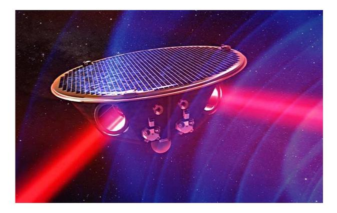
The proposed LISA mission will detect gravitational waves in space using a trio of satellites, separated by millions of kilometers. Lasers will be employed to measure the minute changes in their relative distance induced by impinging gravitational waves. Credit: AEI/MM/exozet; GW simulation: NASA/C. Henze
