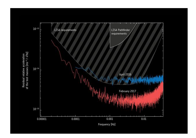
Analysis of the LISA Pathfinder mission results towards the end of the mission (red line) compared with the first results published shortly after the spacecraft began science operations (blue line). The initial requirements (top, wedge-shaped area) and that of the future gravitational-wave observatory LISA (middle, striped area) are included for comparison, and show that LISA Pathfinder far exceeded expectations. Credit: ESA
