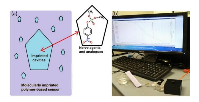
Figure shows (a) the principle of MIP-based sensors, in which unique patterns of the target molecules are imprinted on a polymer-based sensor film and (b) an experiment being carried out using the MIP-based sensor in the laboratory. The sensor response captured by the QCM is displayed on the screen. Credit: National University of Singapore
