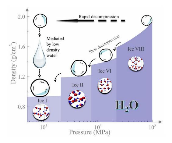
An illustration shows how rapid decompression is the key to observing lowdensity liquid water. Low density water mediates the rapid decompression transition from ice-VIII to ice Ic. Credit: Chuanlong Lin and Guoyin Shen
