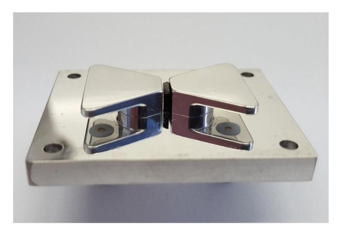
The microwave resonator with the diamond in the middle. Because of the lattice defects, the diamond is black. Credit: Vienna University of Technology
