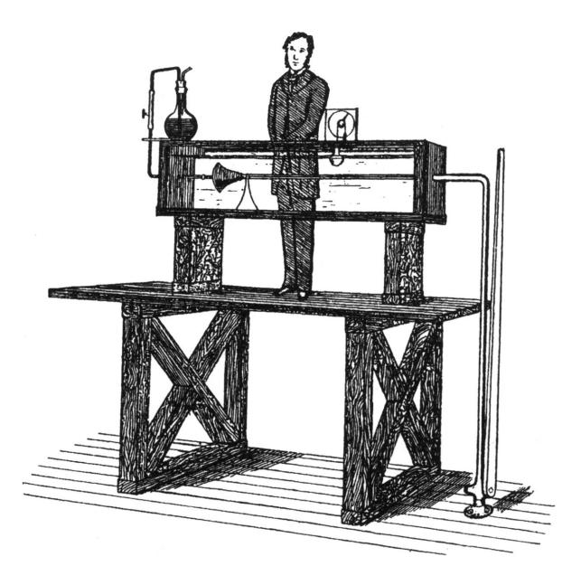
A figure from Osborne Reynolds's 1883 paper, showing Reynolds's assistant standing next to apparatus used to measure friction in different types of flow. Credit: Okinawa Institute of Science and Technology
