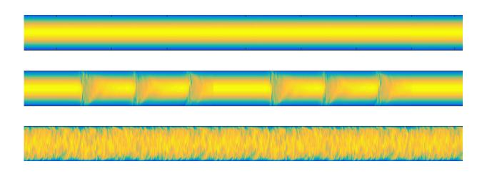
Different types of pipeflow. From top to bottom: laminar, transitional and turbulent. Credit: Okinawa Institute of Science and Technology
