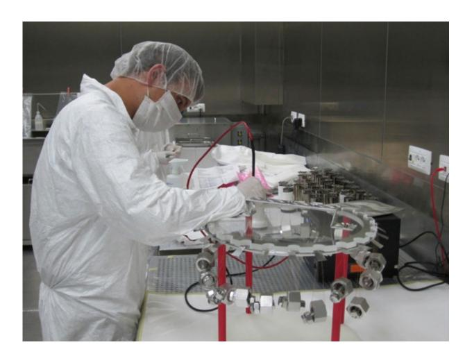
Undergraduate Arthur Kurlej welding the grid electrode onto its support ring inside the radon-suppressed clean room in the underground laboratory at Gran Sasso, Italy. Kurlej's advisor, physics professor Andrea Pocar, says undergraduates were notably helpful in designing and making this component of the dark matter detector there, known as DarkSide-50. Credit: UMass Amherst
