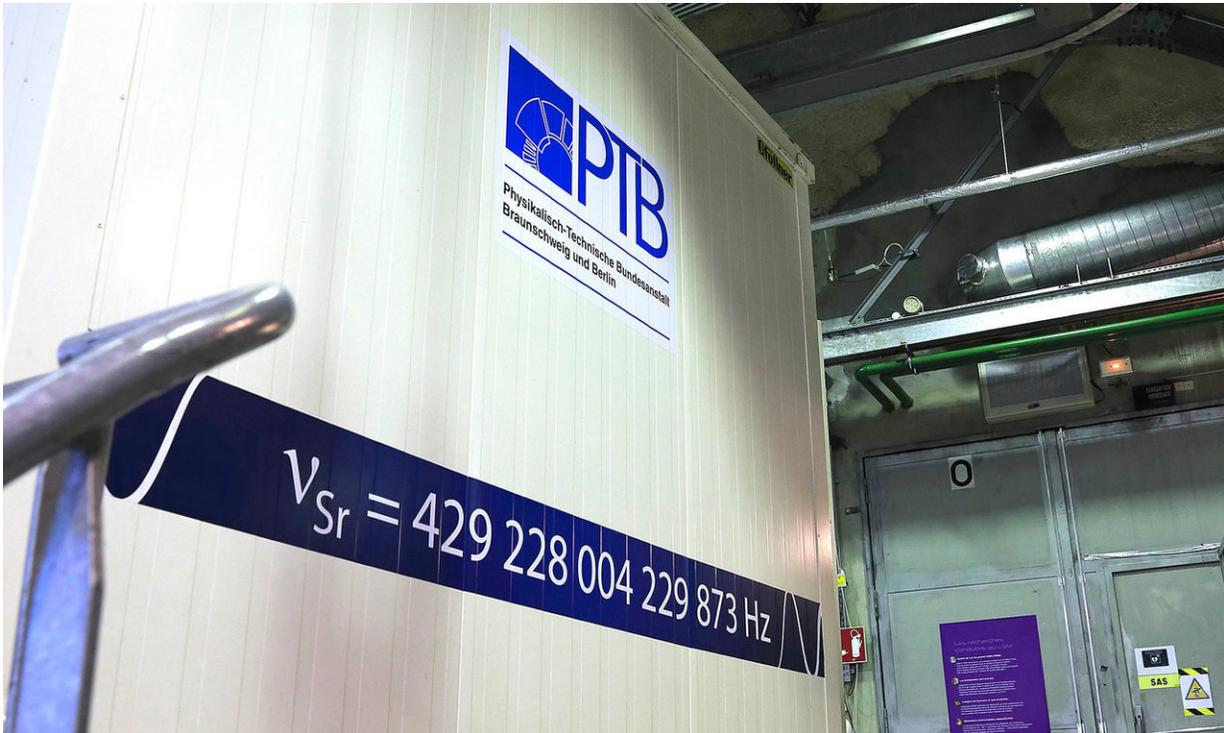
The vibration-damped and temperature-stabilised trailer with PTB's optical atomic clock in the French Modane Underground Laboratory (LSM). Credit: Lisdat/PTB
