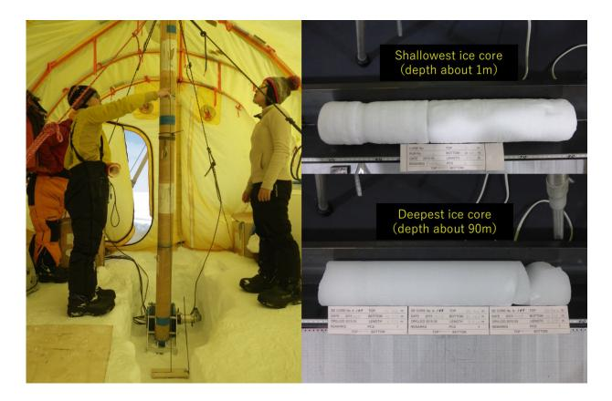
The researchers in the drilling operation (left) and the drilled samples (right). Credit: Hokkaido University
