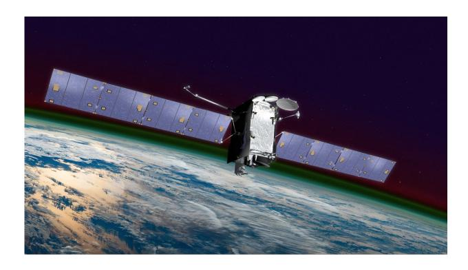
GOLD flies aboard SES-14, a commercial communications satellite (illustrated here), and is the first NASA science mission to fly as a hosted payload on a commercial satellite. Credit: NASA Goddard's Conceptual Image Lab/Chris Meaney
