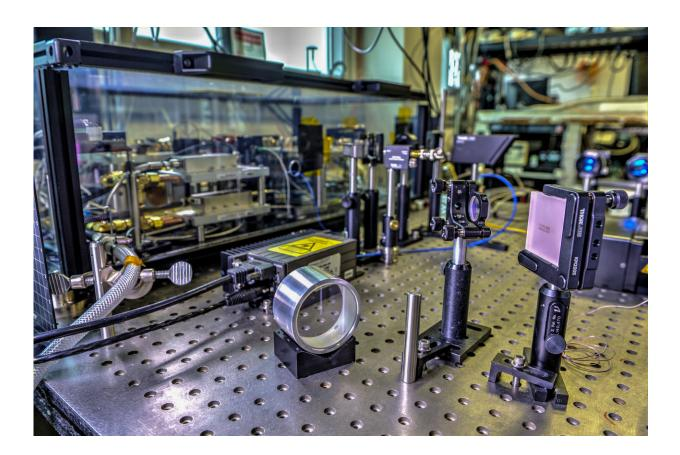
The MARLI instrument breadboard is encased inside the clear case in the background. The cylindrical object in the foreground with the silvery outer shell is the optical etalon used in the lidar receiver. Credit: NASA/W. Hrybyk
