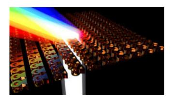
A metasurface with fish-like elements redirects an incoming beam of light into a new direction. Credit: A\*STAR Data Storage Institute
