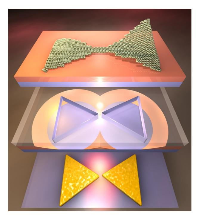
DNA assisted lithography: bowtie-shaped DNA origami is transformed into a metallic nanostructure. Credit: M. Kostiainen
