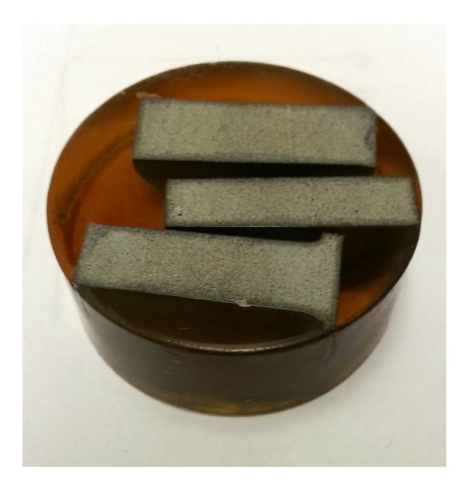
This photo shows cement samples embedded in epoxy ready for microscopy analysis. Purdue University researchers have been working to find the best ratio of mixing cellulose nanocrystals into cement to make it stronger. Credit: Purdue University
