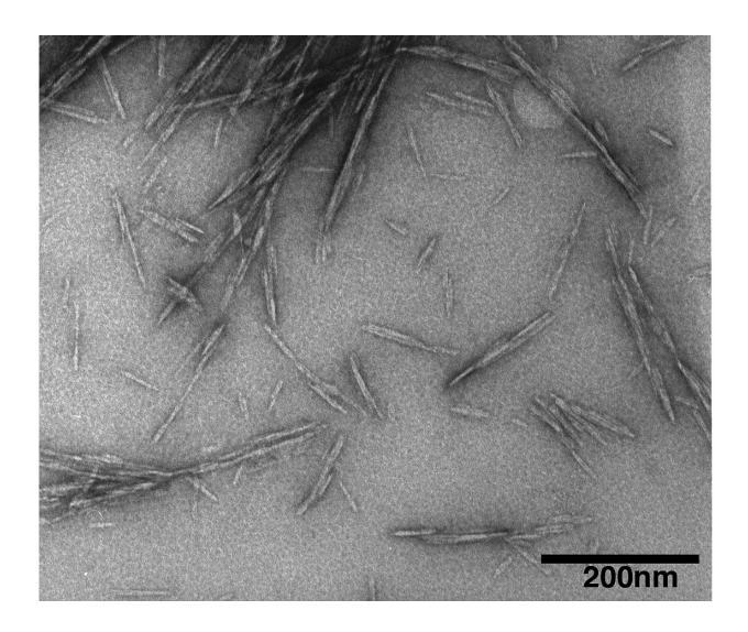
This transmission electron microscope shows cellulose nanocrystals, tiny structures derived from renewable sources that might be used to create a new class of biomaterials with many potential applications. The structures have been shown to increase strength of concrete. Credit: Purdue Life Sciences Microscopy Center
