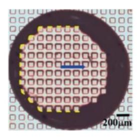
Snapshots of contact line configurations when water droplets slide on surfaces with micro-pillars. Credit: S. Qiao, Q. Li and X. Q. Feng (2018), Sliding friction and contact angle hysteresis of droplets on micro-hole-structured surfaces, *Eur. Phys. Jour. E* 41:25, DOI 10.1140/epje/i2018-11631-x
