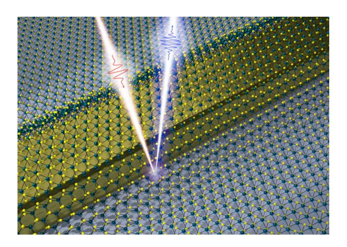
The basic idea of the measurement method: red light hits the surface - blue light is sent back. Credit: Vienna University of Technology
