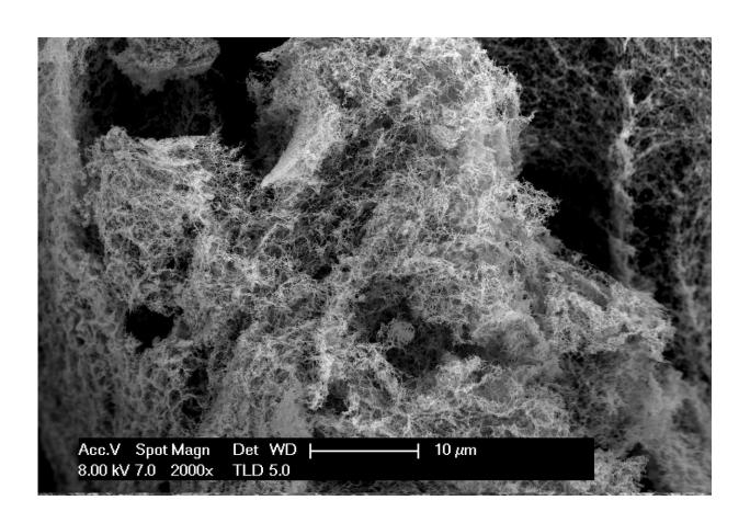
WSU researchers have found a way to create large amounts of inexpensive nanofoam catalysts that can facilitate the generation of hydrogen on a large scale by splitting water molecules. Credit: Washington State University
