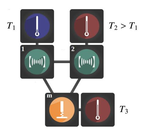
A mechanical system is coupled to two electromagnetic cavities and a heat bath, is proposed as a realization. In this model, the two systems are also connected to their own heat baths. Credit: Shabir Barzanjeh, André Xuereb & Matteo Aquilina
