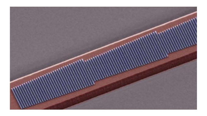
Image of a fabricated device showing four phased antenna arrays consisting of silicon nano-rods of different lengths patterned on the top surface of a LiNbO3 waveguide. Credit: Loncar Lab/Harvard SEAS
