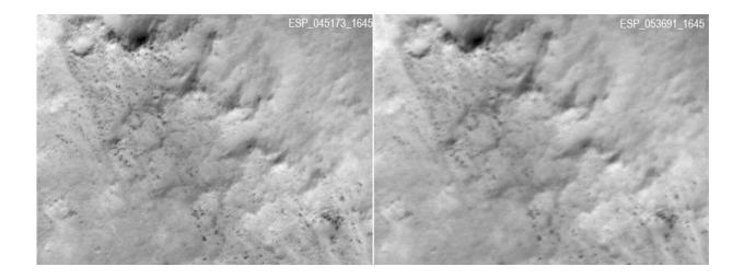
These two frames were taken of the same place on Mars by the same camera before (left) and after some images from the camera began showing unexpected blur. The images are from the HiRISE camera on NASA's Mars Reconnaissance Orbiter. They show a patch of ground about 500 feet wide in Gusev Crater. Credit: NASA/JPL-Caltech/UA
