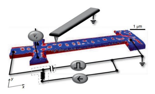
Scheme of the experimental set-up for electrical measurements integrated in an MFM. Blue (red) indicates an attractive (repulsive) force on the MFM cantilever and hence reveals the magnetization in the sample. The sample shape is its actual topography measured by atomic force microscopy. Credit: *Nature Nanotechnology* (2018). DOI: 10.1038/s41565-017-0044-4
