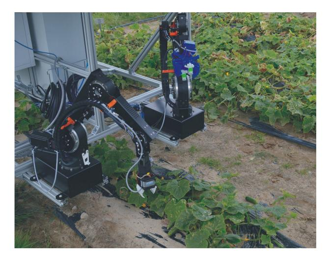
A prototype of the dual-arm robot system during the first field tests. Credit: Fraunhofer IPK
